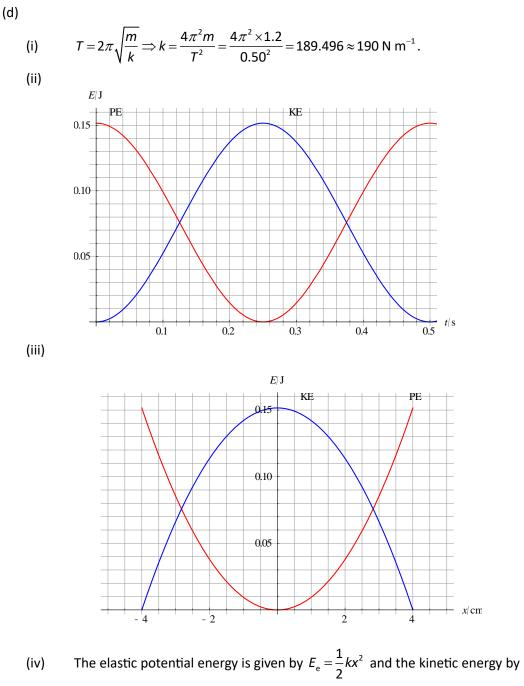
$E_{\rm K} = \frac{1}{2}kx_0^2 - \frac{1}{2}kx^2$  so nothing changes in (iii). In (ii) we have  $E_{\rm e} = \frac{1}{2}kx^2 = \frac{1}{2}m\omega^2 x_0^2\cos^2(\omega t)$ and  $E_{\rm K} = \frac{1}{2}m\omega^2 x_0^2\sin^2(\omega t)$ . The mass quadruples and so the angular frequency halves. Hence the maximum value remains the same but the period doubles. Hence:
